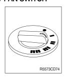
It is possible to control the fan to four steps.
